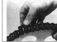
Chain clip installation method
